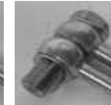
A double banjo bolt requires three copper washers - one each side of each banjo fitting.
