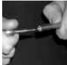
Locate the tip of the fitting just inside the teflon tube and push fitting into the hose.
